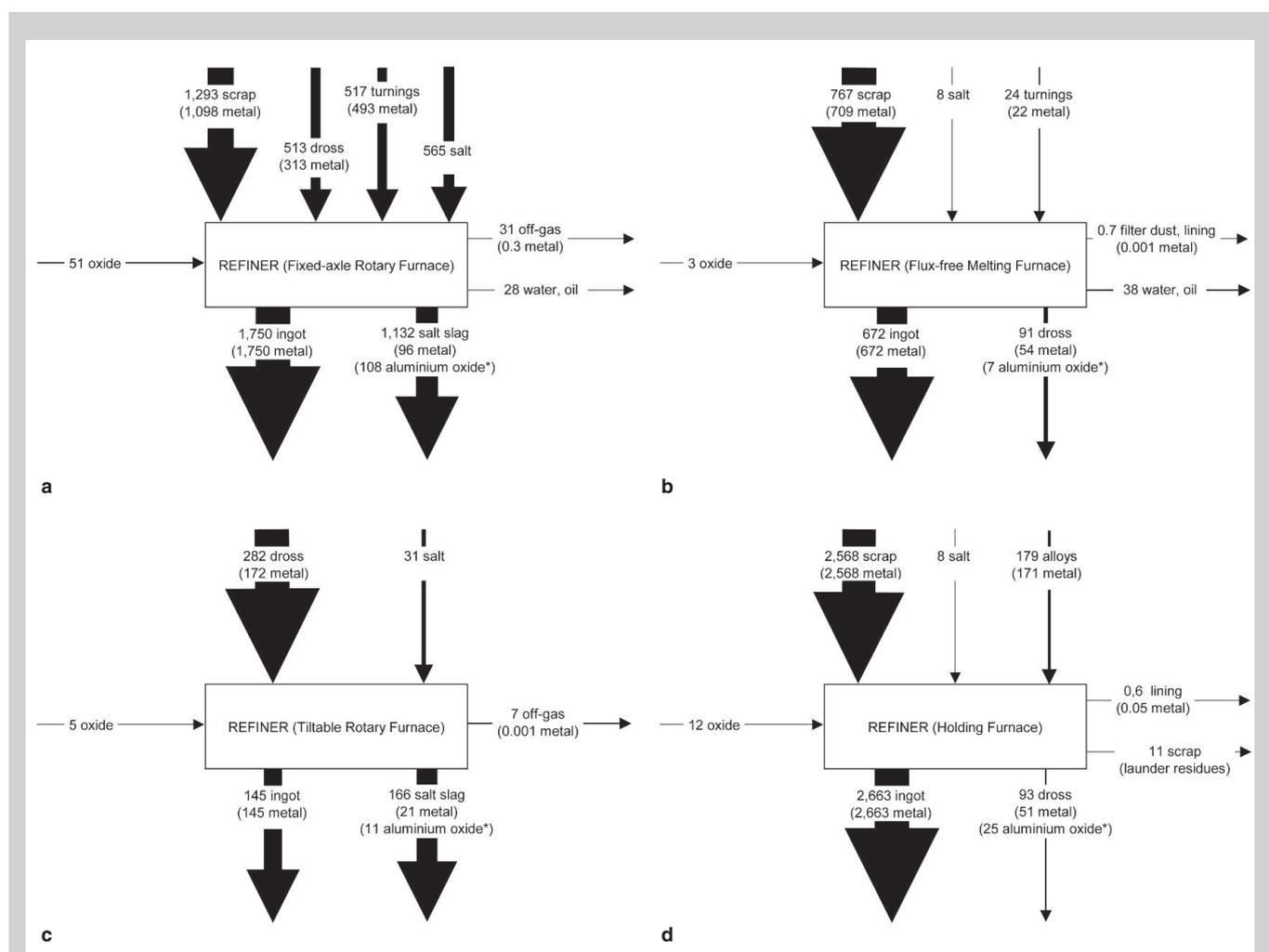
Figure 4. The 2002 EU refiner balance. All units measured in thousand tonnes per year. Quantities shown in parentheses illustrate the content of metal and aluminum oxides within the overall flow. (\*Aluminum oxide formed during the process.) Figures (a) to (c) show the investigated melting furnaces. Figure (d) is the holding and alloying furnace that follows the melting furnaces.
