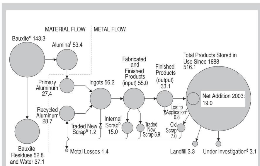
Figure 1. Global aluminum flow.<sup>1</sup> All units measured in million tonnes per year. Values might not add up due to rounding. a—Aluminum in dross; b—not taken into account in statistics; c—such as powder, paste, and deoxidation aluminum (metal property is lost); d—area of current research to identify final aluminum destination (reuse, recycling, or landfilling); e—includes, depending on the ore, between 30% and 50% alumina; f—includes, on a global average, 52% aluminum.
