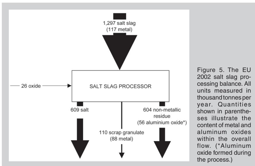
Figure 5. The EU 2002 salt slag processing balance. All units measured in thousand tonnes per year. Quantities shown in parentheses illustrate the content of metal and aluminum oxides within the overall flow. (\*Aluminum oxide formed during the process.)
