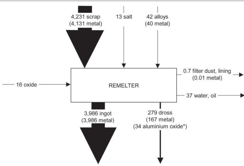
Figure 3. The 2002 EU remelter balance. All units measured in thousand tonnes per year. Quantities shown in parentheses illustrate the content of metal and aluminum oxides within the overall flow. (\*Aluminum oxide formed during the process.)
