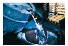
Recycled aluminium poured into ingots for use in new applications
